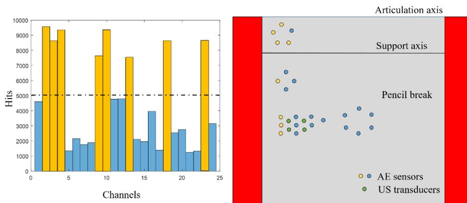
Figure 4. Hits versus channels (left), bottom view of the instrumented slab (right)
