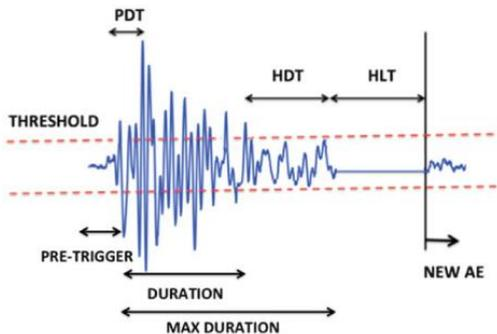
Figure 2. Time domain parameters of an AE waveform (Moradian and Li, 2017)
