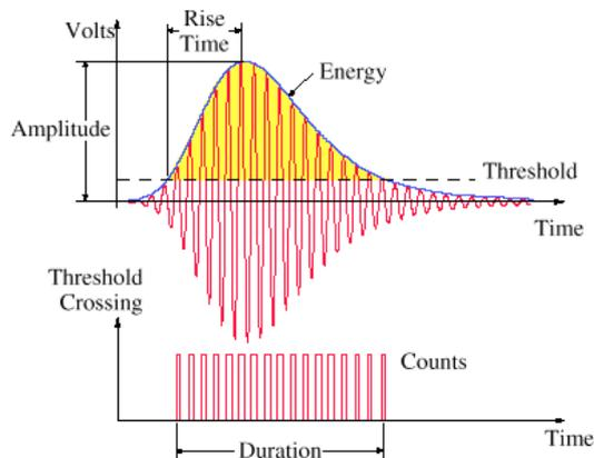
Figure 3. AE common parameters of a waveform (Huang et al., 1998)
