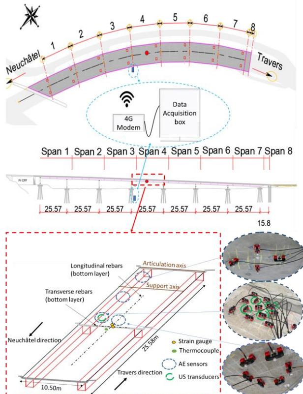
Figure 1. Drawing of the viaduct (plan view and elevation side) - data acquisition system – instrumented slab; dimensions in [m].
