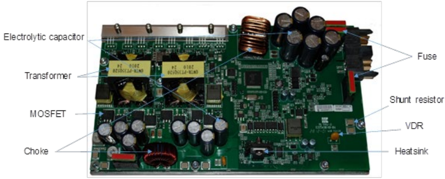
Figure 4-1: Critical power stage subcomponents in a power conditioner utilized in PEMFC (Rastayesh, Bahrebar, et al., 2019).
