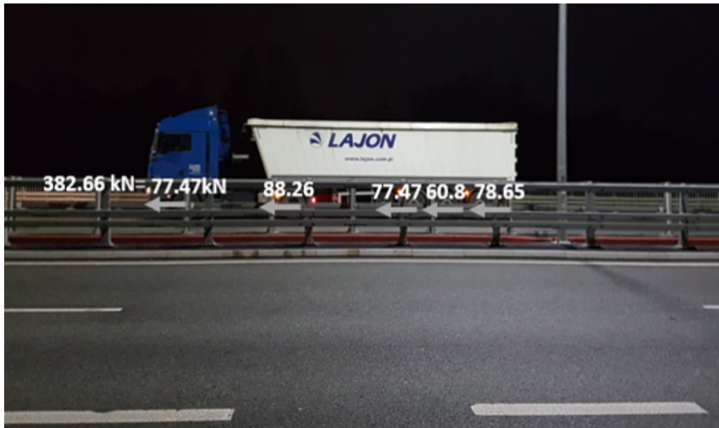
Figure 6.37: Truck (5 axial) used for load test
