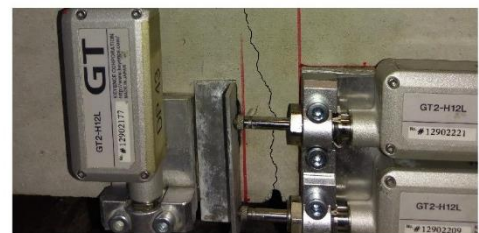
Crack Opening Displacement (COD) measured by LVDTs
