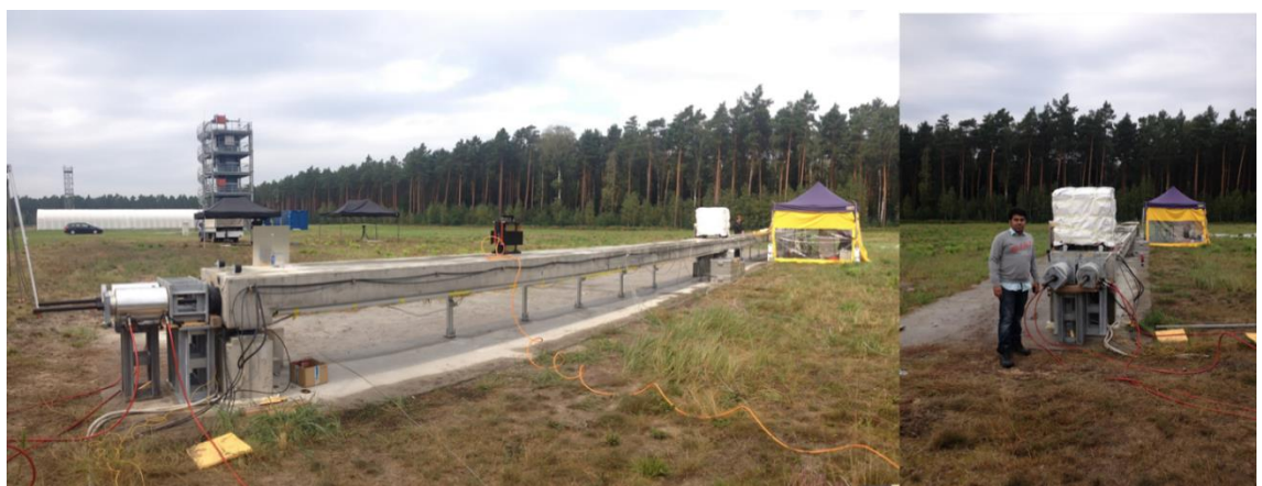
Load test experiment on BLEIB structure.
