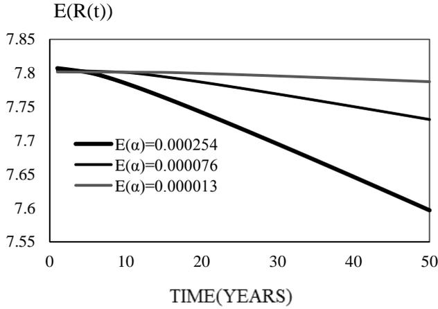
Figure 2. Expected resistance degradation in service life.
