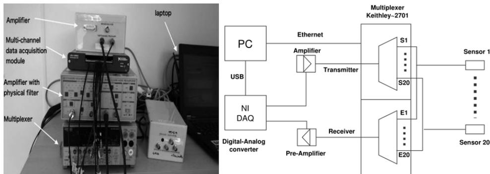
Figure 5. Data acquisition equipment and diagram of the data acquisition system
