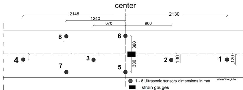
Figure 4. Arrangement of SO807 sensors and strain gauges in the girder
