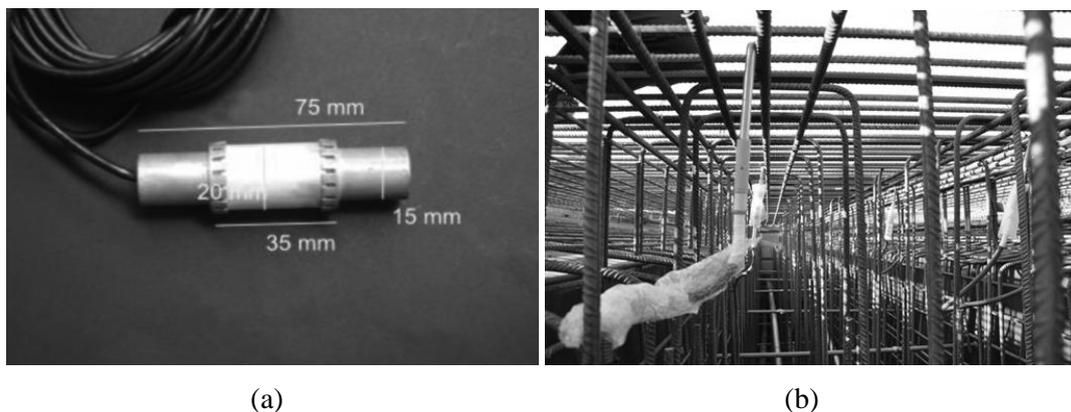
Figure 3. (a) Ultrasonic transducer SO807 (Niederleithinger et al. 2015). (b) Mounting sensor with L-shaped rebar.
