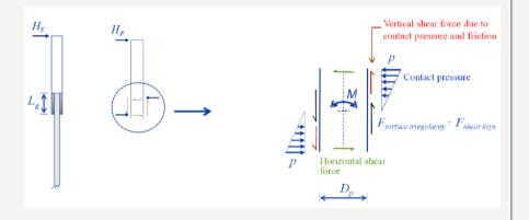
Jacket foundation: sectional forces transferred through compression grout blocks.
