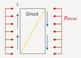
Jacket foundation: compression stress dominated.  $F_{V1Shk}$ Grout
